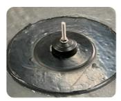
**Step 5**Seal the cuff all around with an UV resistant EPDM sealant.
