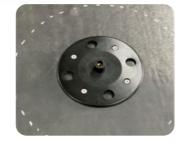
Step 1 Place the black mounting base plate on the roof covering at the desired location. Fasten the mounting base plate with 4 screws. The chosen screw depends on the thickness of the
